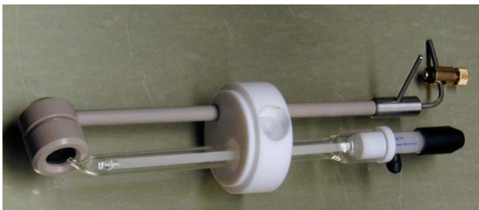
Diskfix with gas diffusion electrode and reference electrode
